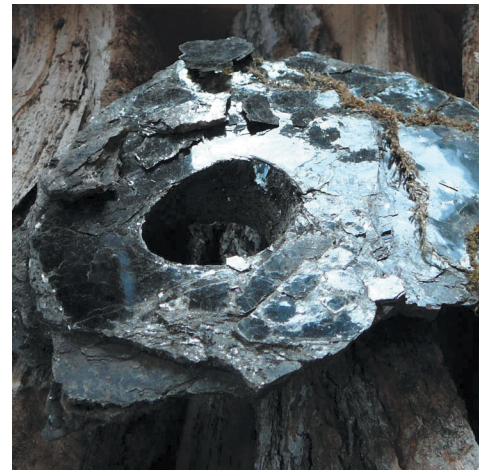
Mica ore with drill hole through the centre
